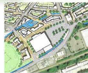
This is a standard ASDA - 55,000sqft net similar to the one in Hulme. The car park is probably too small to be acceptable.
